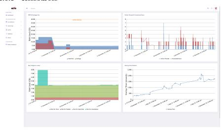
In the left top card you can see a graph showing the Total amount of RAM, as well as the garbage used by the TM1 instance currently selected. A machine maximum, parametrable will help you see how far you are from throttling the machine, and possibly get an out of memory error from TM1.
